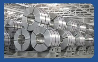
cold rolled steel that has been through additional processing steps, Such as pickling, cold rolling, and annealing. This makes it much harder than mild steel & gives it a better surface finish. cold rolled steel is used for applications in which dimensional tolerances, strength & surface finish quality are critical.
