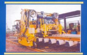
Track Relaying Machine is Four-wheeled Hydraulically driven Machine, which consists of two basic structure units.
