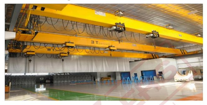
Our Electric Overhead Travelling (EOT) Cranes are engineered for precision, safety, and durability in demanding industrial environments. Designed to handle heavy loads with ease, these cranes offer seamless material handling across manufacturing plants, warehouses, shipyards, and more.
