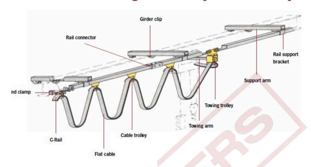
Commonly used in crane systems, hoists, conveyors, and other moving equipment. Their flexible and durable construction makes them ideal for festoon systems, where cables are suspended and guided along a track.
