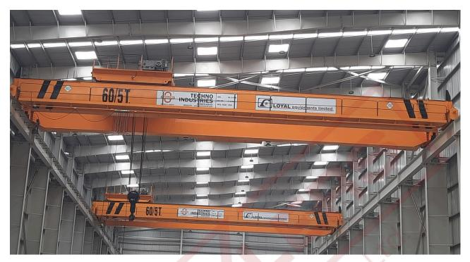
Tacklers Engineering Pvt. Ltd. offers high-performance Double Girder E.O.T. Cranes, meticulously designed for lifting heavy loads and covering longer spans with superior structural integrity and precision. These cranes are ideal for industries requiring frequent, high-capacity lifting and are built with advanced safety features as per IS-3177 and IS-4137 standards.
