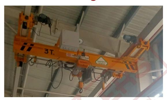
TACKLERS' Underslung EOT Cranes (also known as Underhung Cranes) offer an ideal solution for facilities where supporting steelwork beneath the crane is not feasible. These cranes are suspended directly from the roof structure, freeing up valuable floor space and allowing for smooth, unobstructed material flow—perfect for areas with limited headroom or complex layouts.
