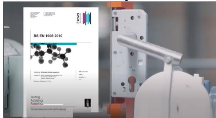
Mortice Lock Life Cycle Test
