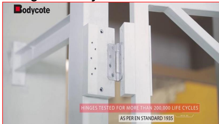
Hinges Life Cycle Test
