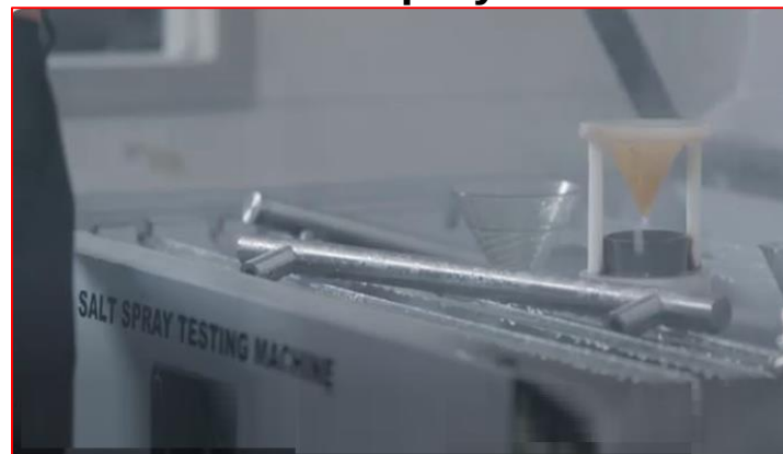
Corrosion Salt Spray Test
