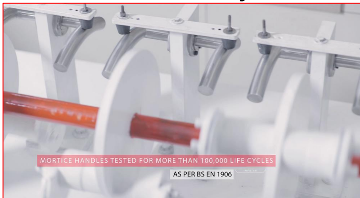
Mortice Handles Life Cycle Test
