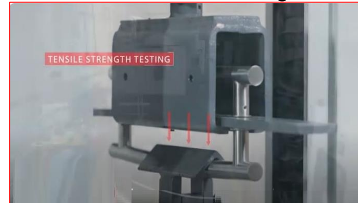
Pull Handle Tensile Strength Testing
