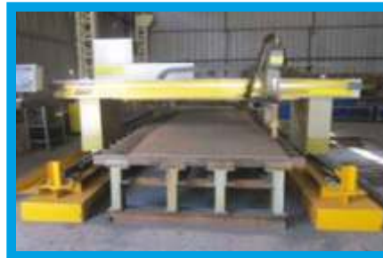
PLASMA MACHINE (CAPACITY - 16 MM THICK)
