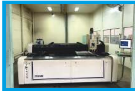
LASER MACHINE (CAPACITY - 8.0MM THICK)
