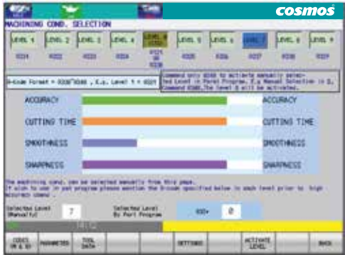
Finish Machining Condition Selection
